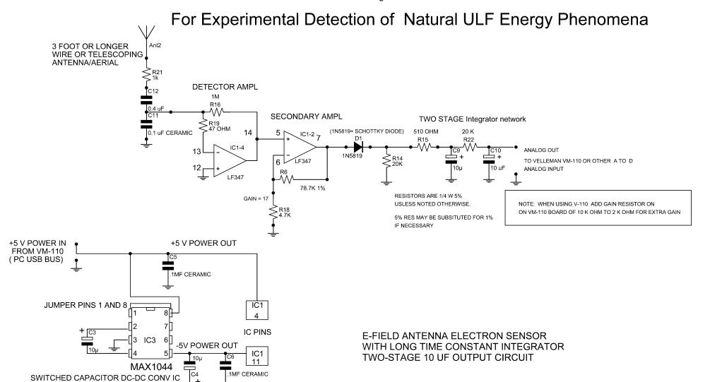
THIS CIRCUIT IS DESIGNED FOR SCIENTIFIC USE IN THE DETECTION OF ULTRA LOW FREQUENCY ELECTRIC ACTIVITY
